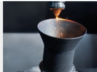
7: Laser construction of the conical funnel
