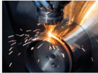
2: 90° swivel: Generation of the flange
