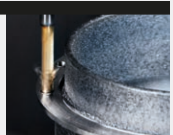
4: Drilling of the flange
