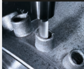
10: Milling of the connectors
