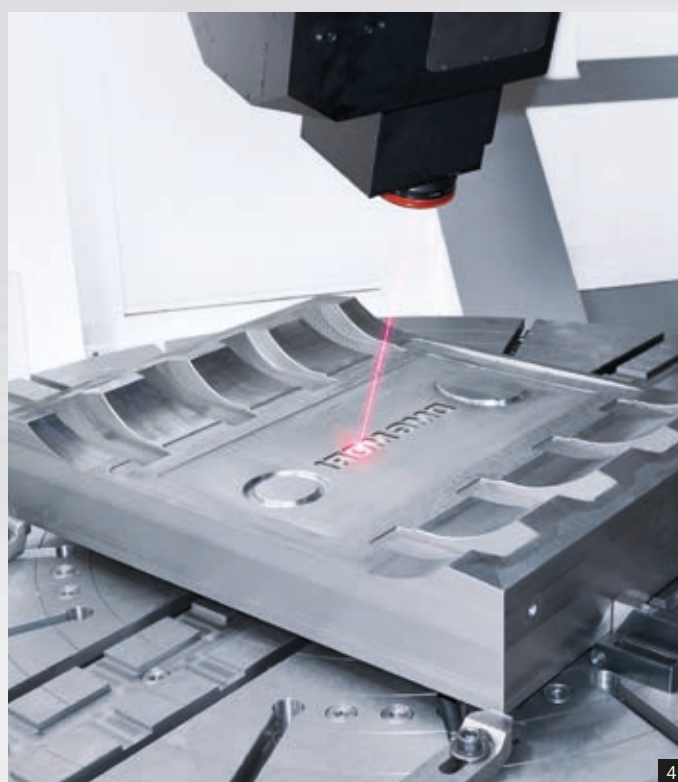
1 + 2: Replacement of the laser scanning head via a special changer device within 10 minutes; interface is the HSK 63 / 100 taper of the spindle 3: Laser texturing of a housing component 4: Surface structures in engine covers
