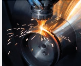
2: 90° swivel: Generation of the flange
