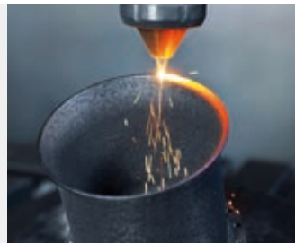
6: Build-up of the crossover section
