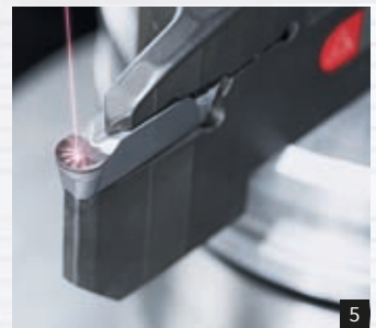
1: Clearly structured working area with optimal workpiece accessibility 2: Massive, consistently stable mineral composite column 3: Precision scanner, CCD camera and measuring sensor 4: High-precision laser machining of demanding, complex geometries on up to 5 axes 5: 5-axis laser machining of a cemented carbide tool with a picosecond laser
