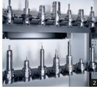
1: Pallet change \leq 30 seconds 2: PH 10|100 linear magazine for the integration of max. 42 HSK tools 3: Option: Retractable drawer for cutting inserts or shaft tools
