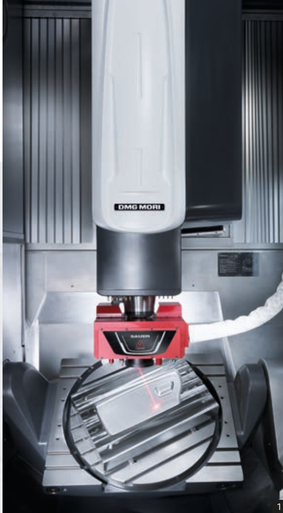
1: Large working area with integrated NC swivel rotary table with perfect accessibility, can be loaded from above by crane 2: Highly stable, compact monoBLOCK® design 3: Flexible integration of a laser scanning head via an HSK interface on the spindle, 5-axis laser texturing of a steering wheel injection mould
