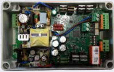
Flex1 ACDC as supply for build in overload protector ex. LIP7 OC #121308, Box size (LxWxH): 180 x 110 x 63 mm
