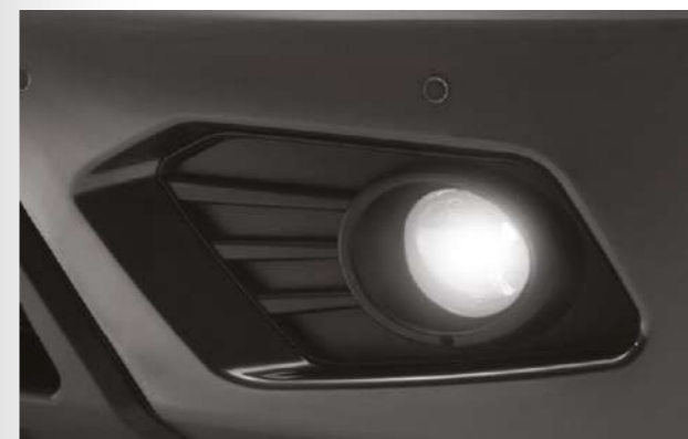
Front fog lights and switchable front parking sensors
