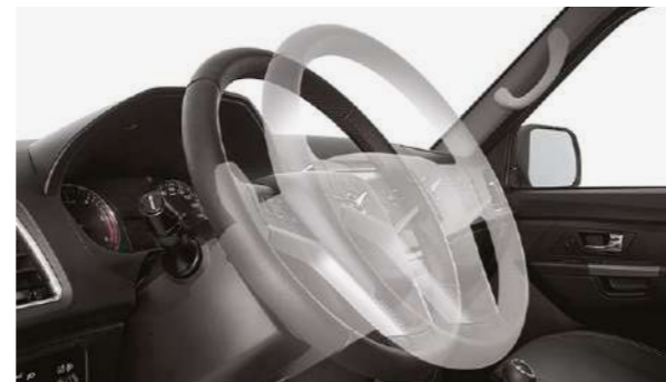
The new UAZ Patriot steering wheel can be adjusted both by tilt angle and height
