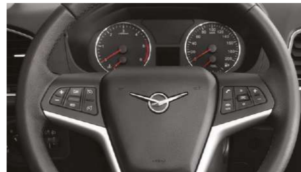
Multifunction steering wheel with cruise control, speed limiter, multimedia system and loudspeaker system controls
