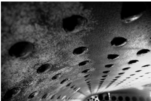
Cover Image - An image of the crown sheet of a mainline, U.S. steam locomotive taken during routine maintenance.
